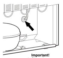
Close the sensor cable opening at the back of the appliance with the sealant provided.
