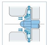
Axial flow suddenly changes into radial flow resulting in flow disturbance and increased bend loss
