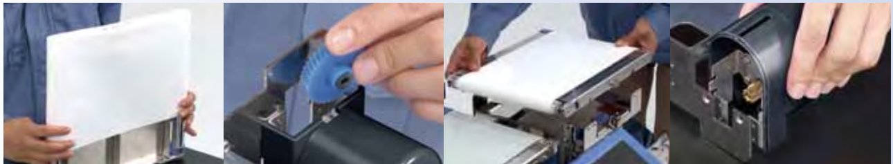
Replacing a belt
