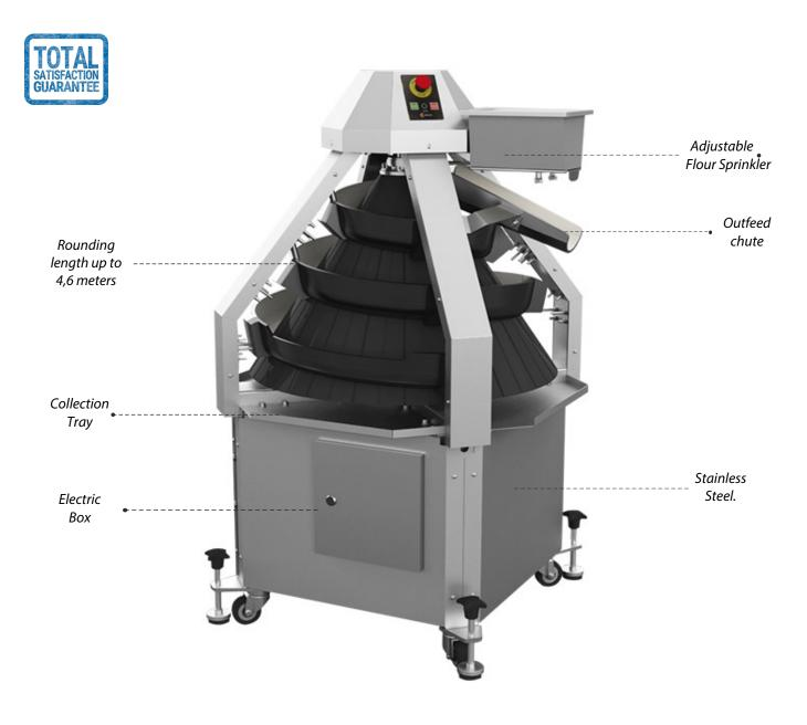
This machine is designed with a rotating cone and adjustable spiral shaped corrosion resistant tracks around it. The dough becomes perfectly rounded while moving from bottom to top in the tracks which are adjustable.
