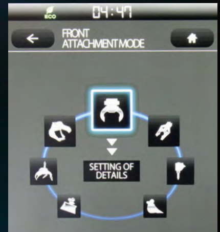
Nibbler is not applicable for Offset boom specification.
