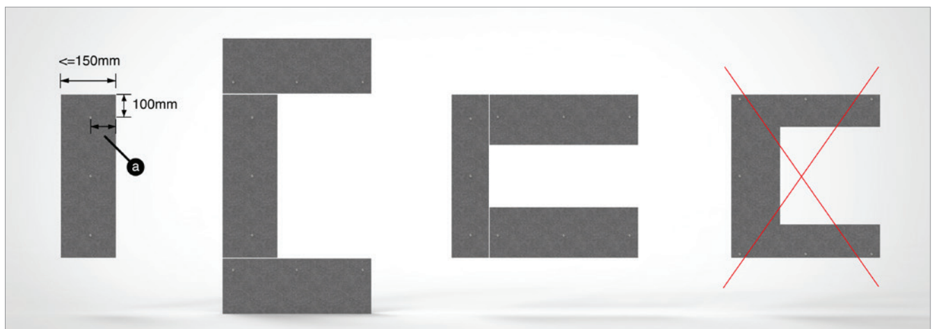
FIGURE 21. Correct installation of Genesis façade boards at windows, doors and openings a: If the small cut-outs are not wider than 150mm, they can be mounted with only one screw in the middle of the board.
