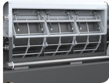
Screen clamping mechanism adopts fast opening design and the screens can be exchanged without any tools.
