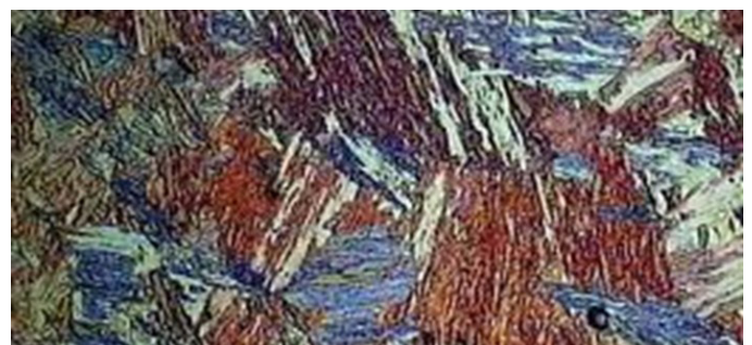
Figure 1: The coarse, acicular crystals of martensite
