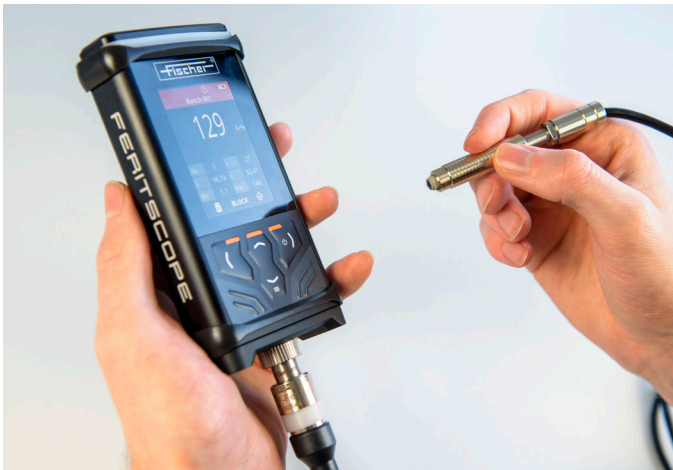
Figure 2: FERITSCOPE® DMP30 with probe D-F-Fe for the measurement of martensite
