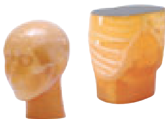
Angiographic CT Head Phantom ACS Head with MECT compatible arteries
