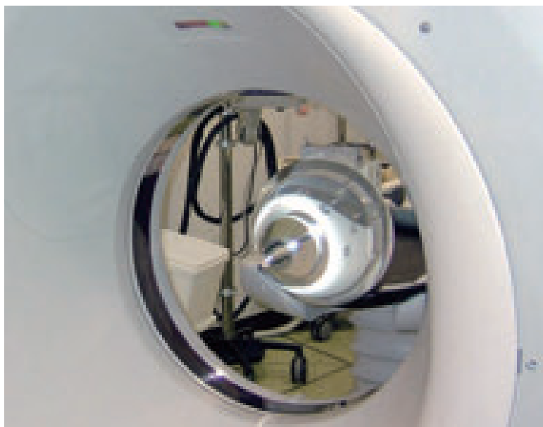
example of CT-AEC with an anthropomorphic phantom
