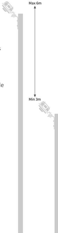
**STEP 2 - DETECTOR ALIGNMENT** – The AGD650 Dual Zone Stop-line Detector should be mounted using the supplied hardware. The optimal mounting angle will change depending on the installation location; aiming the camera to the centre of the area of interest is a good start position. The mounting angle may need to be corrected during commissioning stage of the installation. Ensure the detector is securely fixed and the mounting nut is tight.
