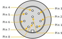
Pin view of bulkhead connector
