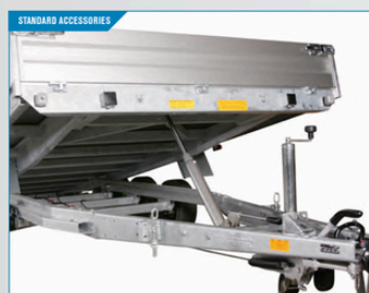
Powerful plunger tip and manual hand pump. Side and stable.
