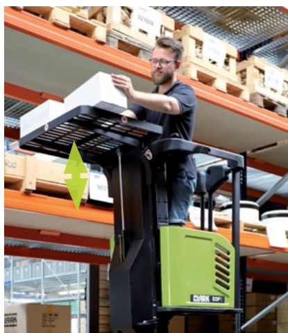
Height-adjustable shelf – adjustment range: 485 mm
