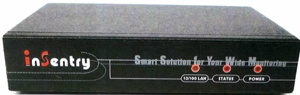
Front View: showing network connect, communication status and power on
