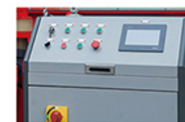
Electric System Intelligent control system with overload protection
