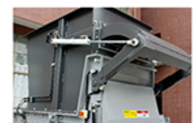
Hydraulic Material Pusher automatic working which can accept contin- uously feeding
