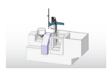
S3 Picker: 3 CNC axes with side axis rotation
