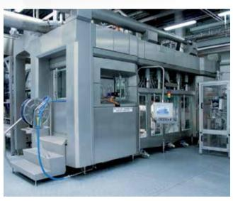
AsepTec fillers have a clear and efficient operator interface with discreet authorization levels so only relevant machine functions will be available to select personnel. The AsepTec flexible linear filler also ensures total aseptic safety to your personnel. To allow effective product tracking and tracing, down to the level of individual bottles, the control system stores production data in an industry-standard database.
