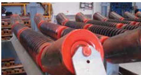
Impact idlers for load support.
