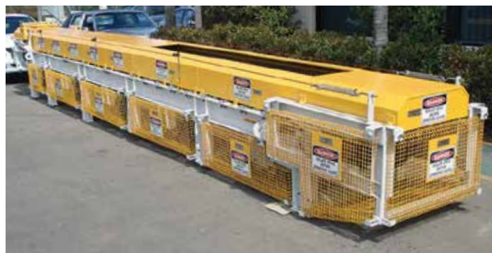
Special belt feeder for sample plant application.
