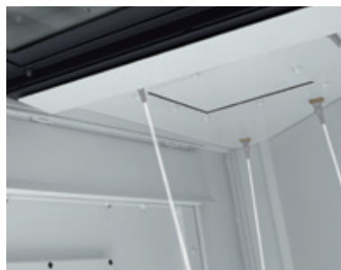
Chip disposal groove
