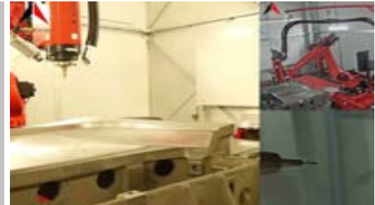
LASER DEPOSITION WELDING WITH WIRE
