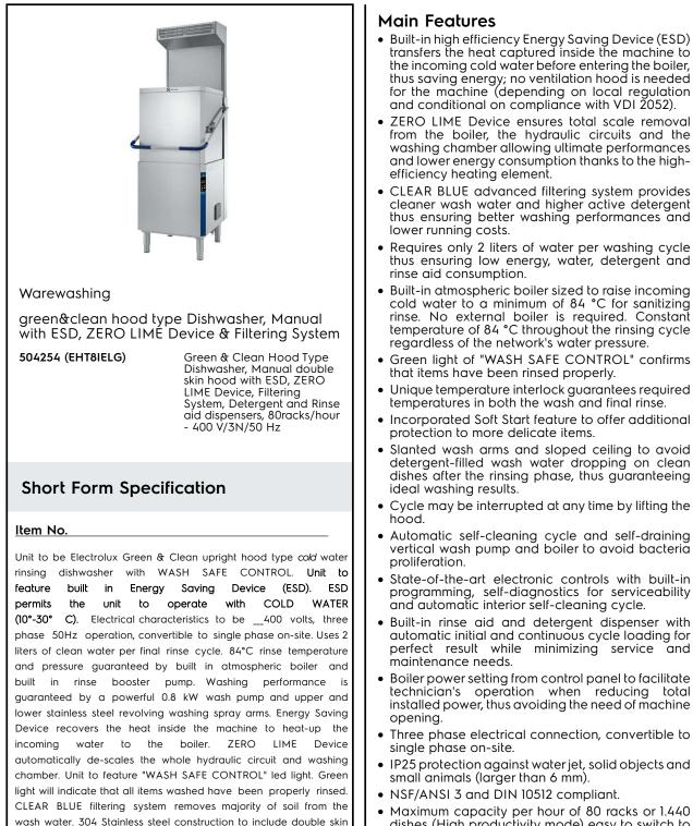
thus saving energy; no ventilation hood is needed for the machine (depending on local regulation and conditional on compliance with VDI 2052). ZERO LIME Device ensures total scale removal
