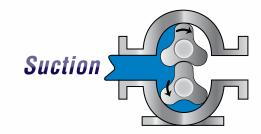
Wright Flow Technologies' rotor lobes rotate around the circumference of the channel in the pump casing. This continuously generates a partial vacuum at the suction port as the rotors unmesh, causing fluid to enter the pump.
