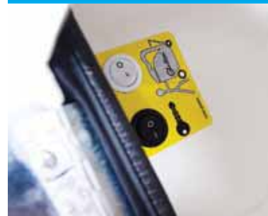
Main ignition switch
