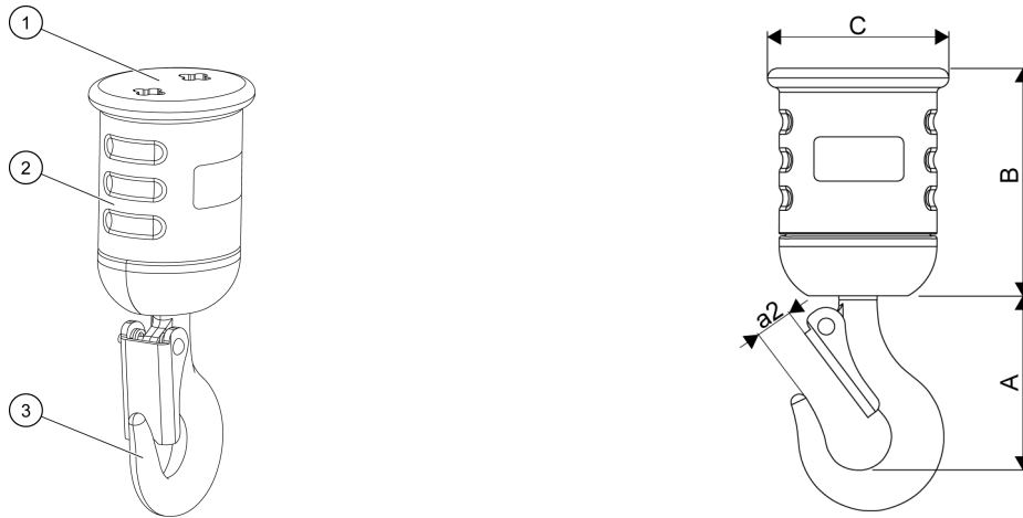
Figure 28. Two-fall (2/1) hook block for frame sizes 02–05
