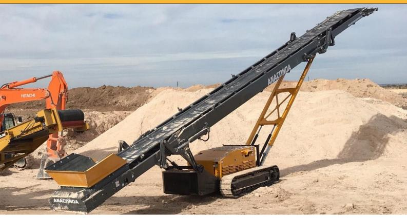
The Anaconda TR Range of Mobile Tracked Conveyors are designed for the Material Handling Sector and aim to reduce production time and save stockpiling costs.
