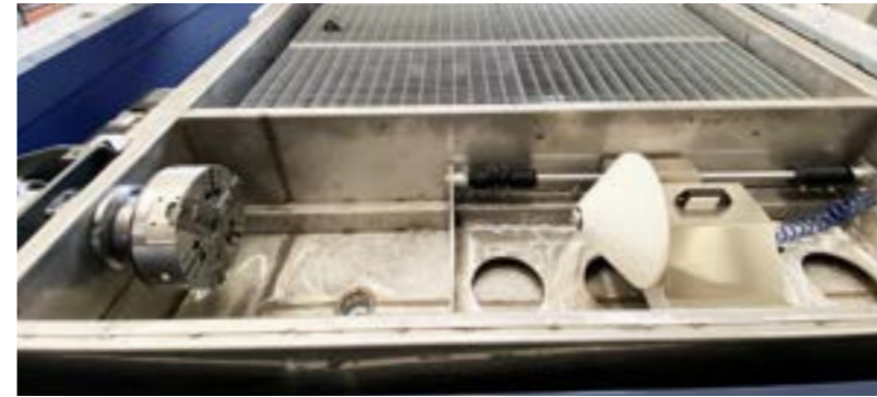
Tubocut • Motorized and CNC controller Mandrel with 3 connection clamps with manual clamping capability • Minimum diameter of the pipe: 64 mm • Maximum diameter of the pipe: 260 mm • Maximum length of the pipe: 1.000 mm • Maximum thickness of the pipe: 45 mm
