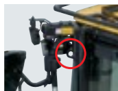
Anchor point of Tie-off
