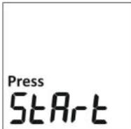
In this **start mode** the configuration of the device can be changed again if required. When plugged into the USB port of a PC, the device is automatically recognized by the liberoCONFIG software and set to "ConF"-mode without the need to press any keys.
