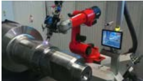
LASER POWDER DEPOSITION WELDING OF A ROLLER
