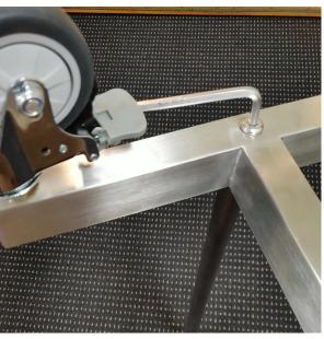
Place the rod with the threaded end and screw into the underside of the rectangular tray frame until all the way in.
