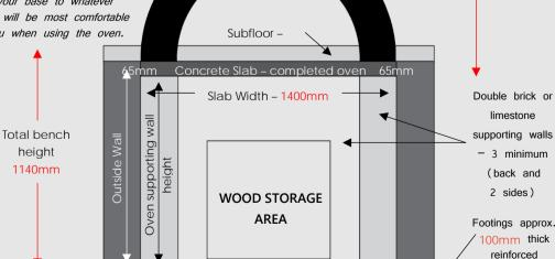
**NOTE** The aim is to have the benchtop level with the oven floor. Therefore the outside wall should be total bench height less thickness of whatever you are using to finish your benchtop eg. tile thickness.
