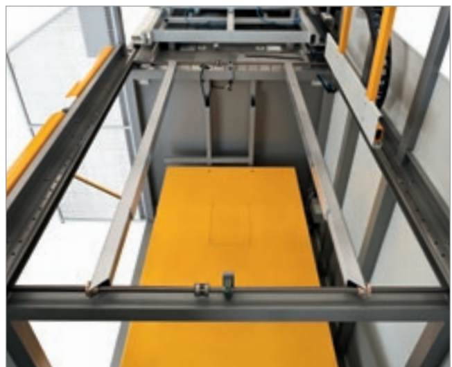
Centring device for automatic sheet positioning
