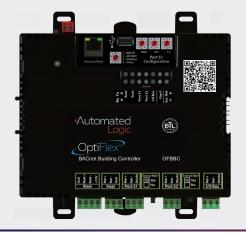
The Automated Logic® OptiFlex™ BACnet Building Controller model OFBBC is a high-performance, BACnet native direct digital controller and BACnet router. As a component of the WebCTRL® building automation system, this controller provides comprehensive control of connected equipment.
