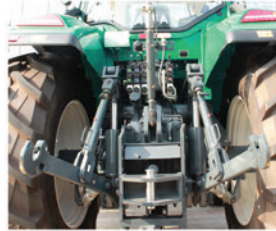
Strong backend with heavy lift capacity draft control linkage.
