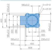
Mounting option: Floor Protection class: IP54/67
