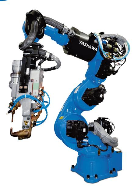
The 7-axis MOTOMAN VS100 robot provides unique, slim design which optimizes automotive spot welding applications. It is the industry's first 7-axis spotwelding-robot which offers a highly flexible range of motion. This robot can be placed in close proximity to work pieces and other robots to create flexible, high-density layouts, eliminating multiple stations and resulting in shorter production lines and smaller spot welding work cells.
