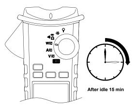
The meter can work again by turning it on from the OFF position.
