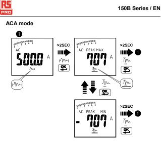
In PEAK HOLD mode, the meter is activated to save the positive peak value and negative peak value. Positive peak value is displayed in PEAK MAX mode. Negative peak value is displayed in PEAK MIN mode.
