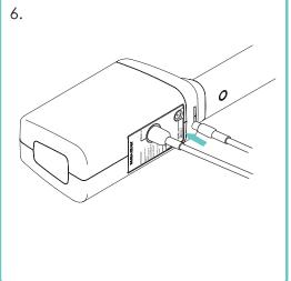
6. Plug the 12V Power Supply cable from the power supply into the 12V port at the rear of one of the monitor Head-Units only.
