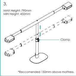
Lift clamp lever to unlock, adjust monitor height to required level and lock by pushing clamp lever down.
