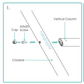
1. Place the crossbar section onto a flat surface and screw crossbar to vertical column using supplied screw and M5 Allen Key, then place cap on hole.
