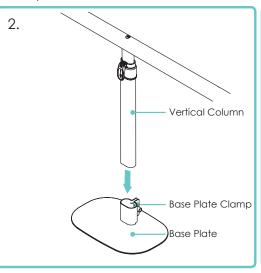
2. Place the Vertical Column into the Base Plate clamp and tighten screw firmly with supplied M8 Allen Key.
