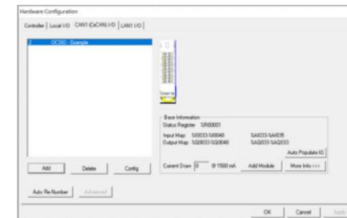
8. Now modules can be added via the "Add Module" button. As I/O modules are added the Input Map, Output Map, and Current Draw are updated, showing the accumulated I/O Module Information. More details regarding each module can be viewed via the "More Info" button.
