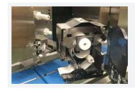
Label change/replenishment is very quick thanks to Ishida's unique label cassettes. Operators can prepare all labels for the next production run in advance. Changing the cassette on the printer takes just a few seconds.
