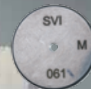
Worn SV Orifice Spraying Systems Co.: 10% increase in flow rate
