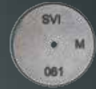
Worn Orifice Competitor: 20% increase in flow rate
