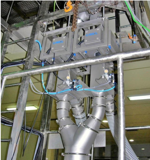
METAL SHARK® GF Twin Installation for particularly high flow rates.
