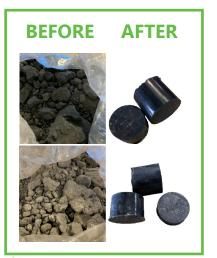
The new BTF-P line of briquetting machines is the line dedicated to grinding sludge, machining waste from sharpening, polishing or grinding operations, consisting of carbide powder mixed with oils or emulsions of oil and water. They are classified as hazardous and must be handled appropriately.
