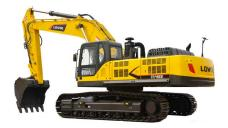
Lovol ES and ER technology is adapted for the hydraulic system through confluence & energy recycling, thus the working efficiency is substantially improved by 8% compared to the same size machines of other brands. KPM (same as Hitachi) pumps means proven and trusted operation for maximum hours.
