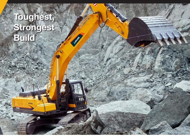
The Lovol 48 tonne Excavator features a Cummins Engine, one of the most reliable, trusted and fuel efficient engines available. KPM hydraulic system with pilot oil operated joysticks for precise control. Many of the problematic electronic items are eliminated and with the toughest heavy duty construction the Lovol FR480E is a machine that saves you down time and costly repairs.
