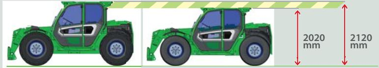
TF30.9 and TF33.7 telescopic handlers are also available in the "Low Profile" cab version, which allows the machine's height to be reduced by 10 cm without compromising on the cab's internal size and operator's comfort. Optimised for work in environments with limited heights as poultry farms, underground car parks, mines.
