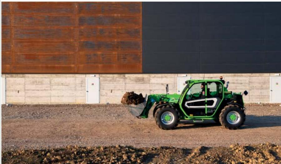
The active boom suspension system (BSS) is available as an option, which protects the load during transfer and maintains a high level of driving comfort on rough terrain. The suspension is automatically deactivated at low speed (below 3 km/h), for boom maximum precision and power.
