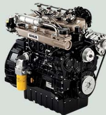
The P27.6 models are equipped with the new 75 HP (55 kW) four-cylinder KOHLER KDI2504TCR 2,500cc engine. The engine complies with Stage V anti-pollution regulations with DOC (Diesel Oxidation Catalyst) and DPF (Diesel Particulate Filter) system.
