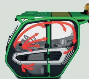
The air conditioning system is completely new and has been developed according to automotive standards, halving the warm-up and cool down times so as to ensure the optimal temperature even in extreme weather conditions. The inlet vent is placed on the side of the cab, away from potential sources of dust and dirt to maximise the service life of the filters. Inside there are eight vents, three of which are dedicated to defrosting the windscreen, for optimal climate comfort.
