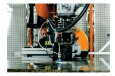
Farnese and BACA Systems introduce the most reliable and lowest cost SawJet Cutting System to the stone industry. Robo SawJet is a high-production dual table SawJet that integrates both a high-pressure abrasive waterjet and 20HP direct-drive saw. Robo SawJet can save customers 70 on labour and 20 on material cost.
