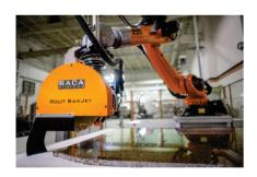
Robo SawJet is waterproof and dustproof. That makes it maintenance proof in the harsh environment of the stone manufacturing. By placing the robot between the two tables, Robo SawJet provides a small footprint for a busy granite fabricators production floor.
