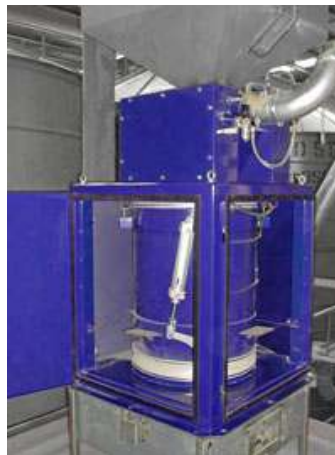
IPW200—Gravity fed with single position radial catch gate
