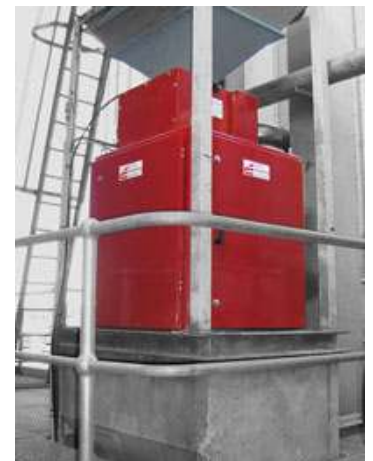
IPW150—Gravity fed with radial catch gate and discharge door
