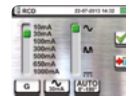
Selection of RCD type and tripping current
