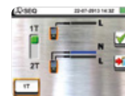
Selection of measurement type of phase sequence
