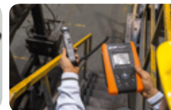
Lux measurement with accessory HT53/05.
