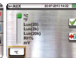
Selection of measurement type with external probe
