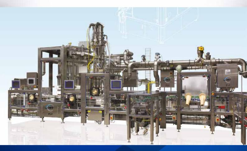
Versatile and hygienic units designed to fill by vacuum, volume and time-fill – or even a combination of these variables.
