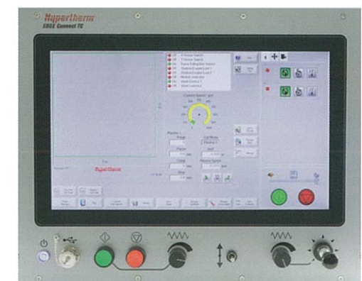
■ A hardware operator's console with switches for start, stop, program and manual speed control, raise/lower torch and joystick is included for easy operation.
