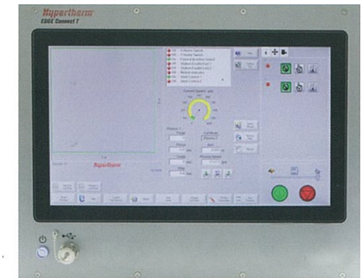
■ Integrates the EDGE Connect CNC into an industrial enclosure with a 495 mm (19.5") touchscreen.
