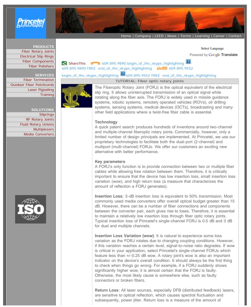
reflection accruing in an optical system. A -45 dB reflection is equivalent to 45 dB return loss. While return loss as high as 60 dB can be achieved with singlemode fibers even for multi-channel FORJs, the typical figure for multimode is around 40 dB.
