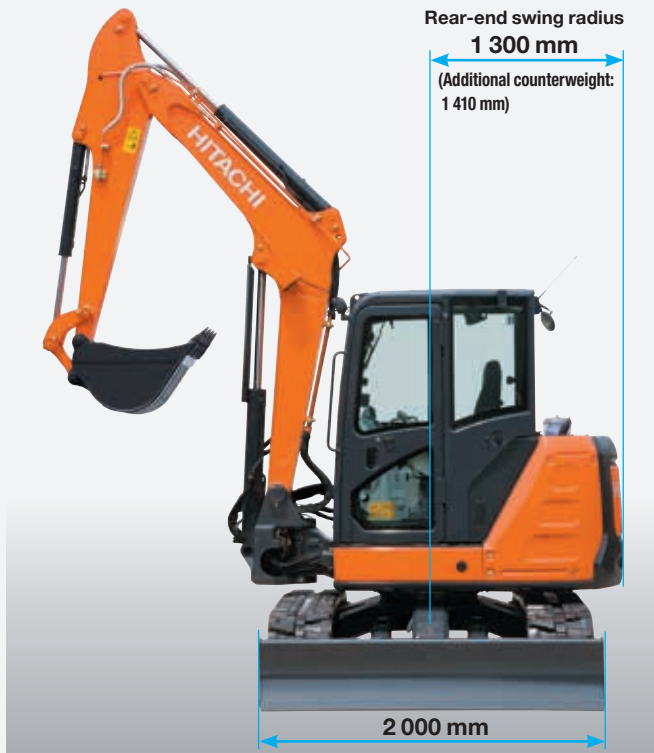
Shown equipped with 1.85 m arm, extra piping, and pre-cleaner.
